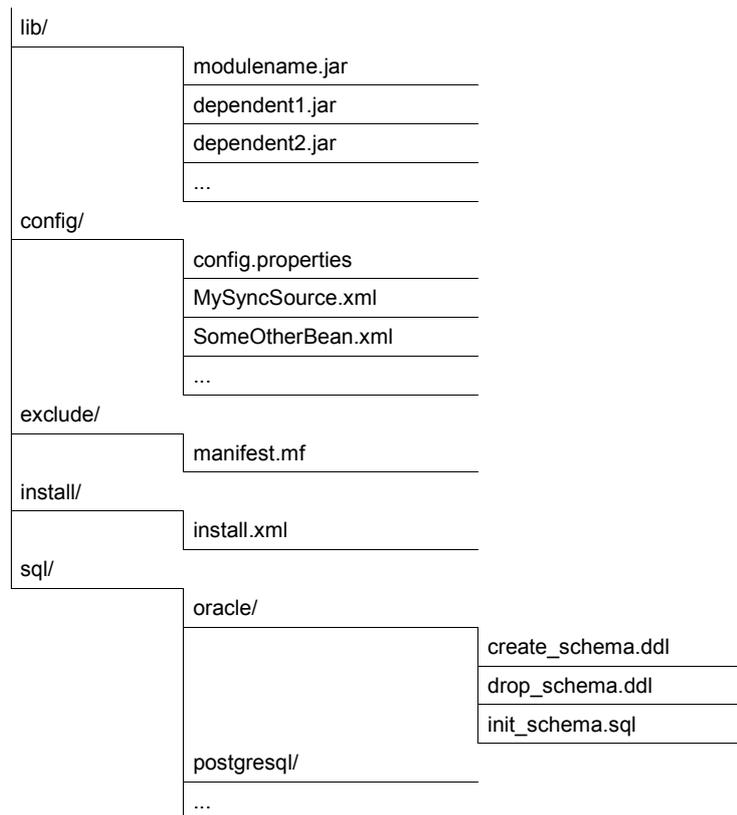
Figure 10: Module package structure
