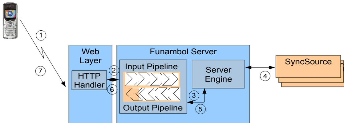
A synchronization session starts with the client device sending a first SyncML message to the server. The request then follows the flow described below:
